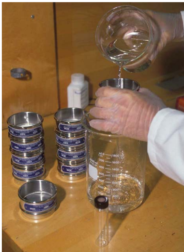
Figure 56. Sieving samples and collecting sample portion for chemical analyses.
