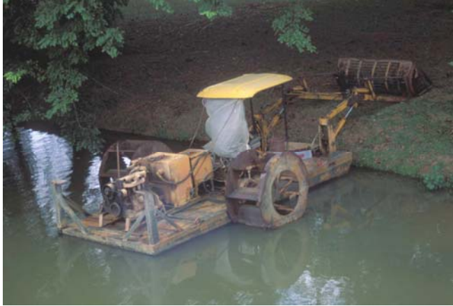
Low-tech aquatic plant harvester, Singapore Figure 31. Aquatic plant harvesting in treatment ponds.
