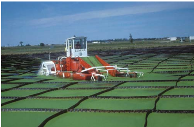
Aquatic plant culture system harvester at stabilization pond (Lemna Corp. photo)
