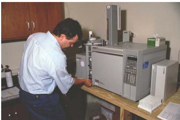
Gas chromatograph with mass spectrograph for the analyses of stormwater organic compounds (mostly PAHs and phthalate esters)
