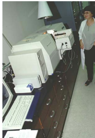
Graphite furnace atomic absorption spectrophotometer for low level heavy metal analyses (detection limits of 1 to 10 \mu\text{g/L} commonly needed, especially for filterable forms)
