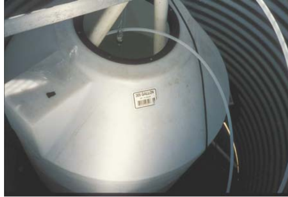
Pilot-scale detention pond for pre-treating water before bioassay tests
