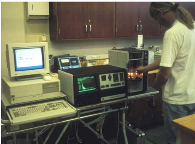
Coulter Counter used to measure particle size distributions
