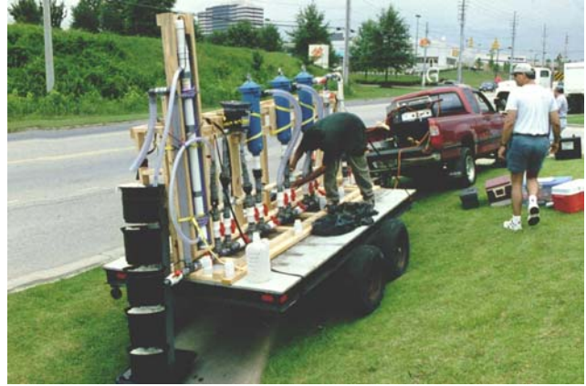
Pilot-scale tests using different cartridge filters, along with sorption materials, disinfection, and aeration, Birmingham, AL
