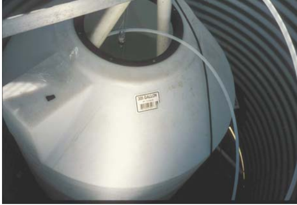
Pilot-scale detention pond at Lincoln Creek side-stream toxicity test lab, Milwaukee, WI
