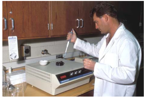
Microtox unit to conduct relative toxicity tests on sample portions
