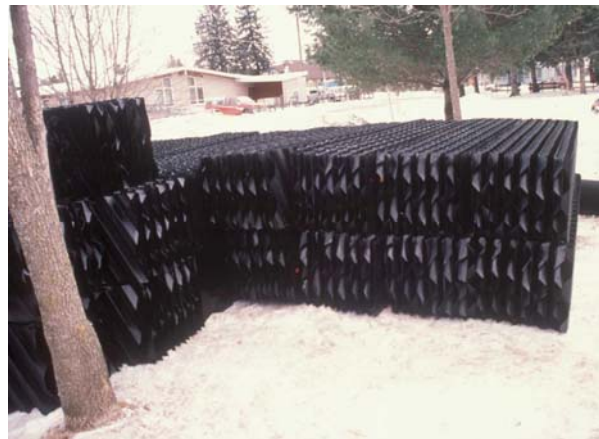
Inclined-tube settlers at Minocqua, WI, MCTT
