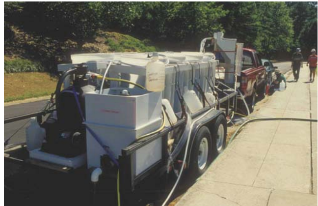
Pilot-scale filtration setup for post-sedimentation treatment tests
