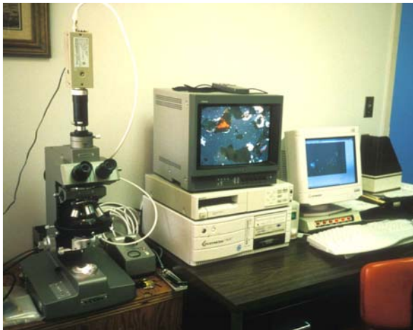
Polarized light microscope to identify sources and characteristics of stormwater particulates
